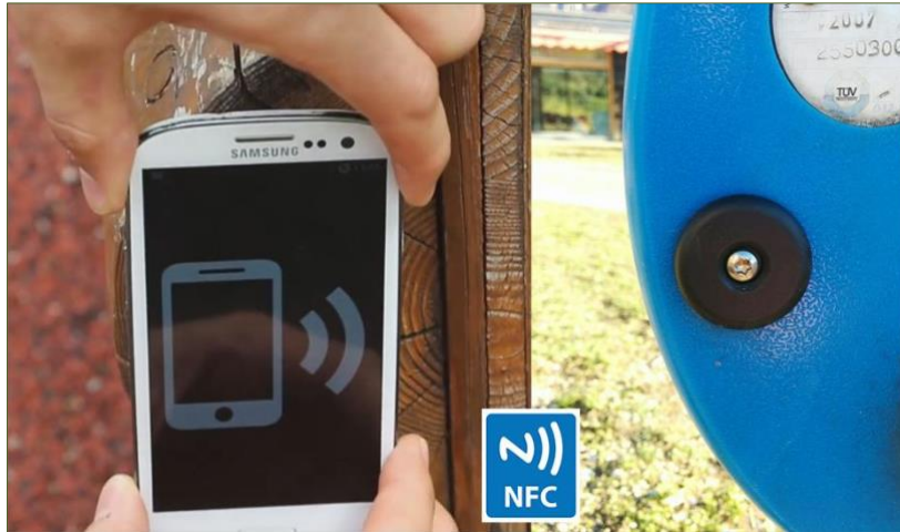
Fig. 8: Registration of inspections of playground equipment using NFC tags.
